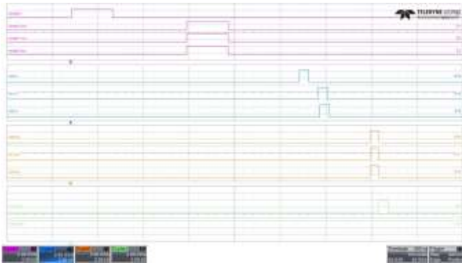
Figure 25. Cables: 1, 6 and 10 mt in length. In addition to the aligned STROBEs, the TRIGGER stream check-up signals coming from the modules are added before and after the time alignment. The last down is the global trigger signal that is output from the summation and majority algorithm
