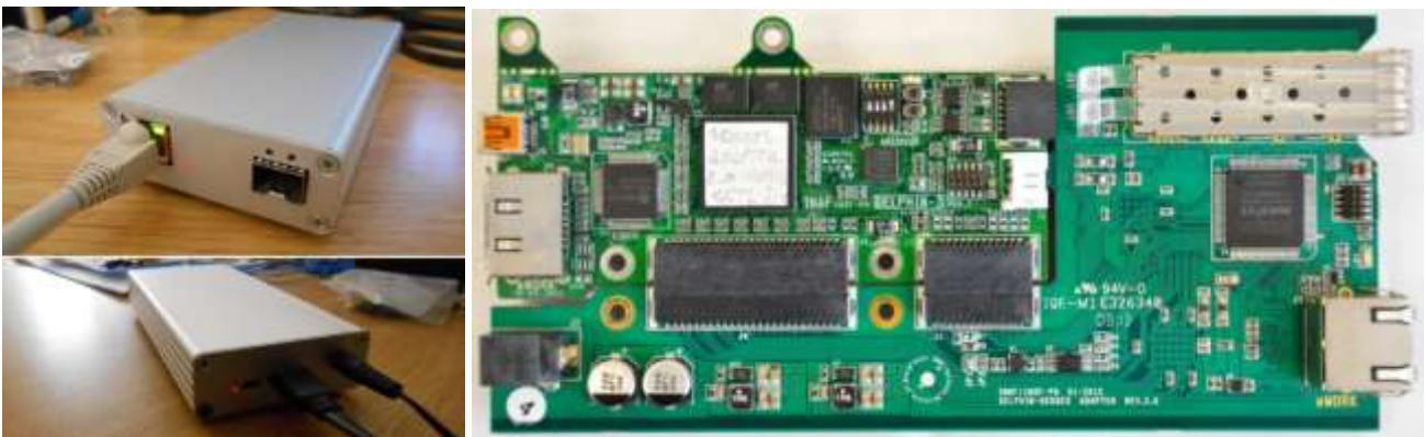
Figure 8. I/O interface (left) and the DELPHIN board (top center) integrated into the GAW I/O interface
