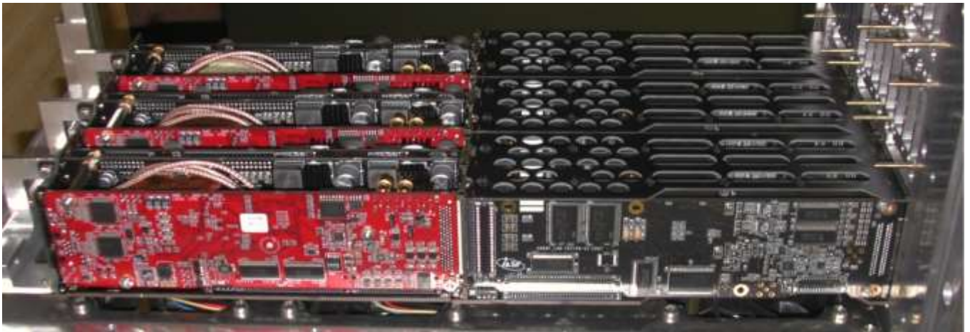
Figure 2. A row of 3 adjacent acquisition modules, in a 3 x 3 focal plane
