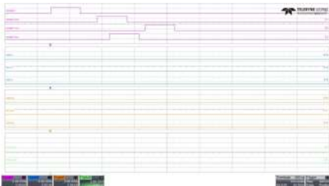
Figure 23. Cables: 1, 30 (fiber optic + SFP) and 10 mt in length. STROBEs of modules 1-3 before time alignment
