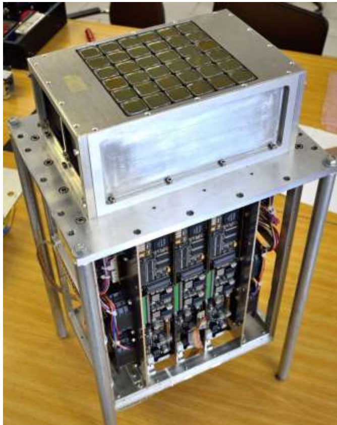
Figure 30. GAW focal plane complete with 6 x 6 phototubes (36 units of 8x8 MAPMT = 2304 total pixels)
