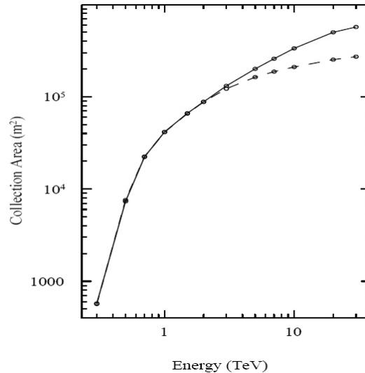
Figure 1: Collecting area of the GAW telescope array vs energy for on-axis Gamma Ray events. Solid line refers to a focal plane detector with a large FoV of  $24^\circ \times 24^\circ$  while the dashed line refers to a small FoV of  $\sim 5^\circ \times 5^\circ$ .
