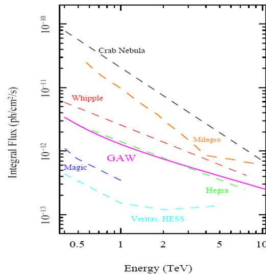
Figure 2: The sensitivity limit ( $5\sigma$ ) detection of GAW (solid line) for Crab-like point sources in 50 hours observations. The flux of the Crab Nebula and the sensitivity of other TeV experiments (dashed lines) are also shown for comparison. The Milagro sensitivity is for 1 year of observation.
