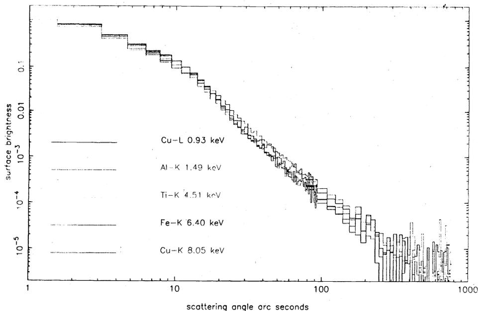
Figure 7: JET-X Mirror Off-Axis Scattering at 4 energies
