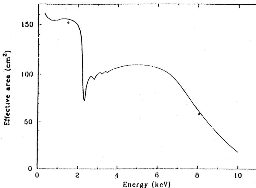
Figure 1: Theoretical JET-X effective area (one telescope). The two points represent the measurements on JET-X FM2 at 1.5 and 8.1 keV.
