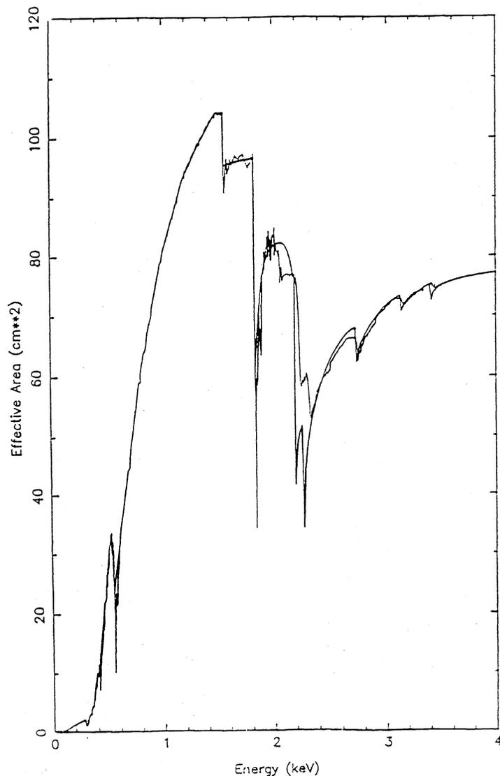
Figure 4: The all-up effective area for the JET-X telescope. Two curves are given - one for which the detailed edge structure was input from direct measurement (thin line) and the other in which the edge shapes were calculated using classical cross-sections (thick line).
