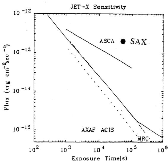
Figure 8: JET-X On-Axis Point Source Sensitivity
