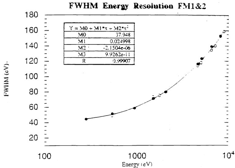
Figure 3: CCD Spectral Resolution
