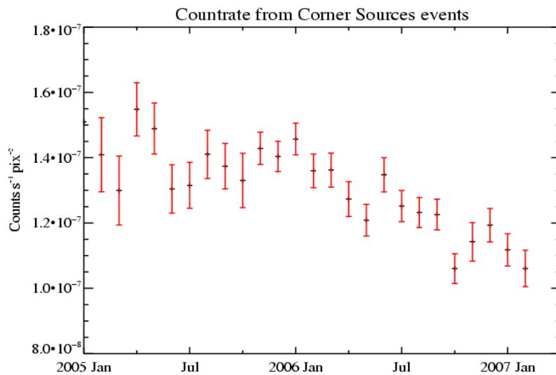
Fig. 3. The count rate of the events from the spectral line at 5.9keV has decreased since the start of the mission. These events are produced by K- $\alpha$  emission of the  $^{55}\text{Fe}$  radioactive corner sources with a half-life of 2.7 years.
