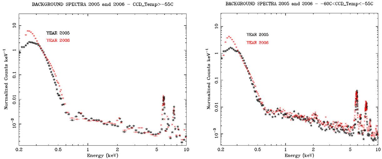
Fig. 2. Background spectra extracted at CCD temperature ranges of  $T > -55\text{C}$  (left) and  $-60\text{C} < T < -55\text{C}$  (right) from year 2005 and 2006. The spectra have been extracted by selecting event grades 0 to 12 only. For both temperature ranges, the comparison of the spectra shows an increase of low energy background events during 2006 compared to 2005.
