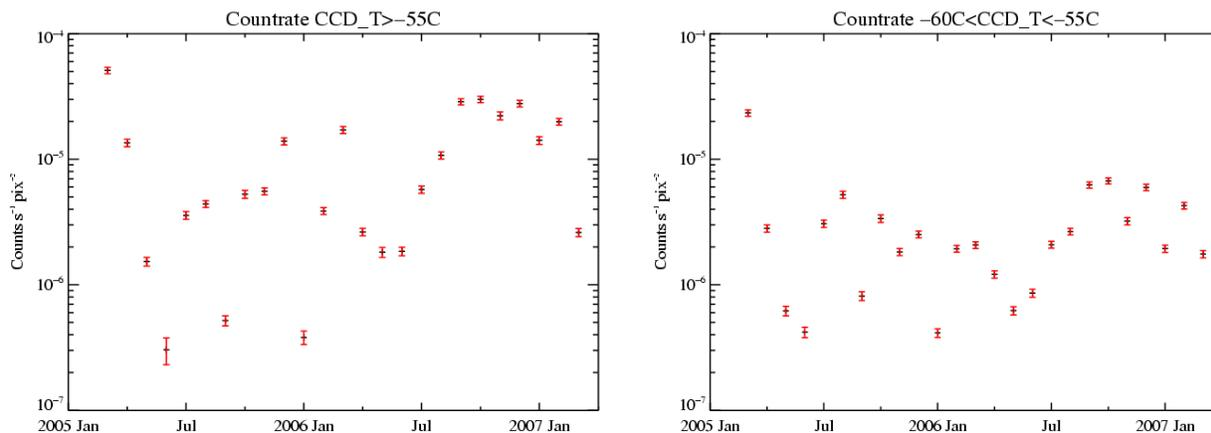
Fig. 1. Background count rate since the start of the mission at CCD temperatures  $T > -55\text{C}$  (left) and  $-60\text{C} < T < -55\text{C}$  (right). The count rate is lower at colder CCD temperatures. The comparison of early data points with count rates at later times does not indicate an overall increase in the background level.
