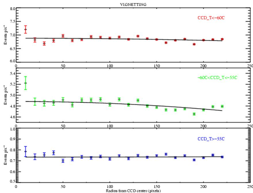
Fig. 6. Number of background events per pixel included in annular regions of increasing radii from the center of the chip at *COLD*, *MEDIUM* and *HOT* temperature ranges. The black lines are the best linear fit of the data with a constant component as the instrumental background and a vignettted component to account for the cosmic X-ray background.
