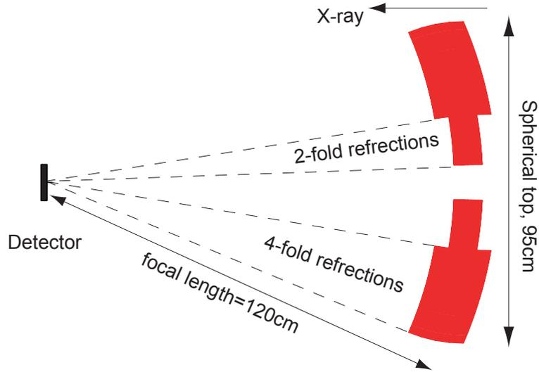
Figure 2. Schematic design of the mirror system and the overview of the WFS. The telescope adopts a spherical top.
