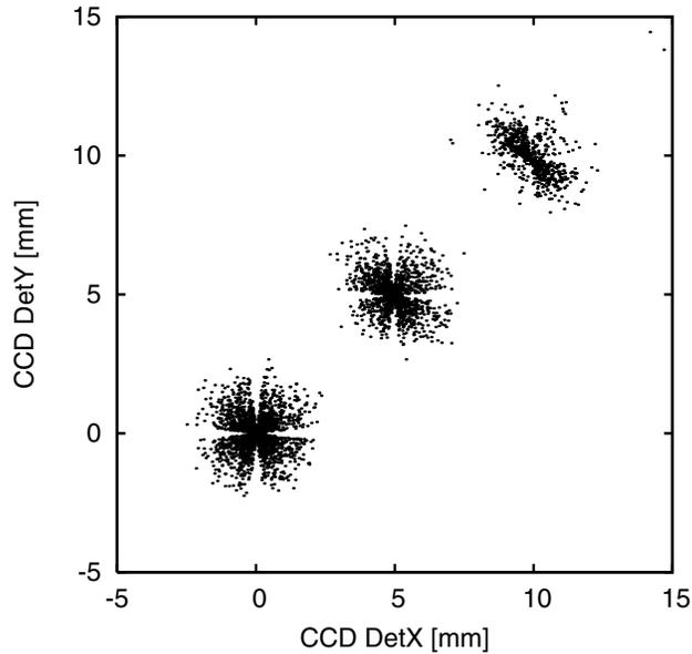
Figure 5. The simulation of the mirror response for an on- and off (20 and 40 arcmin) point source. The housing of telescope assumes the same design as SUZAKU satellite.
