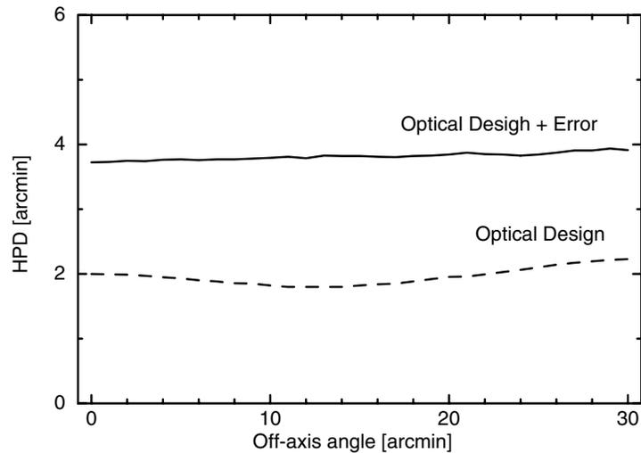
Figure 6. The calculated position resolution of the off-axis angle for the telescope. The dashed line presents the ideal design. The solid line is a prediction including the mirror positioning error  $\pm 8\mu\text{m}$ .
