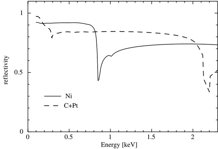
Figure 4. Calculated reflectivity of composit mirror at grazing angle of 1.0 degree. The reflectivity curves are Ni (solid line) and C + Pt (dashed line) in figure.
