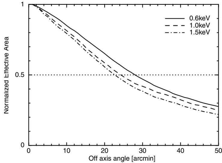
Figure 8. The vignetting curve with off-axis angle at 0.6, 1.0 and 1.5 keV.
