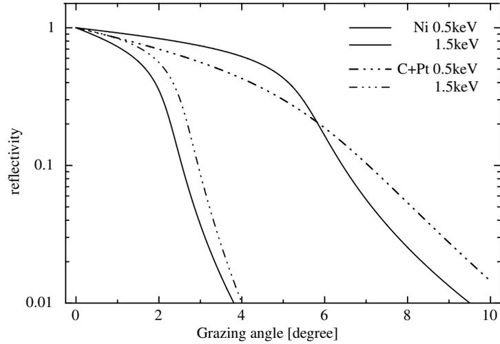
Figure 3. Calculated reflectivity vs. incidence angle for 0.5 and 1.5 keV X-rays.
