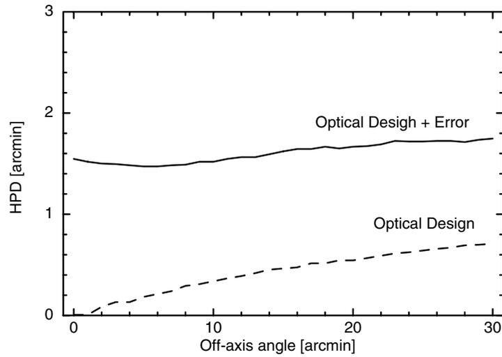
Figure 9. The calculated angular resolution of the off-axis angle with positioning error for the telescope using Wolter-I optics. The dashed line presents the ideal design.
