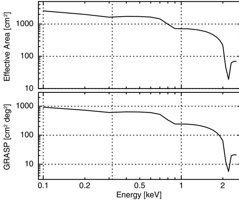
Figure 7. The calculated effective area [cm<sup>2</sup>] of the telescope in the upper panel. In the lower panel is the grasp [cm<sup>2</sup> degree<sup>2</sup>] with detector 15×15mm<sup>2</sup>.
