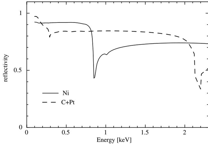
Figure 4. Calculated reflectivity of composit mirror at grazing angle of 1.0 degree. The reflectivity curves are Ni (solid line) and C + Pt (dashed line) in figure.
