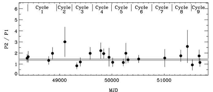
**Fig. 4.** The P2/P1 flux ratio of the Crab pulsar in the 1–3 MeV energy interval as a function of time. The  $\pm 1\sigma$  uncertainty interval assuming a constant ratio is indicated by the shaded region. The P2/P1 ratio is consistent with being constant.
