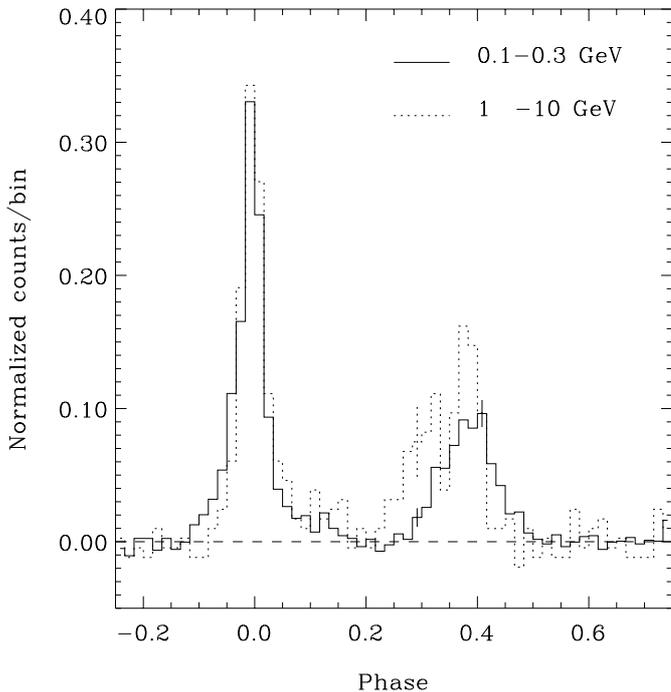
**Fig. 12.** EGRET pulse profiles (60 bins) using CGRO EGRET Cycle 0-VI data: 1-10 GeV, dotted line; 100-300 MeV, solid line. The profiles are normalized to their emission in P1. Typical error bars are indicated for both profiles. A clear increase is visible in the LW2 phase interval (0.25-0.32) for the 1-10 GeV energy interval with respect to the 100-300 MeV interval.
